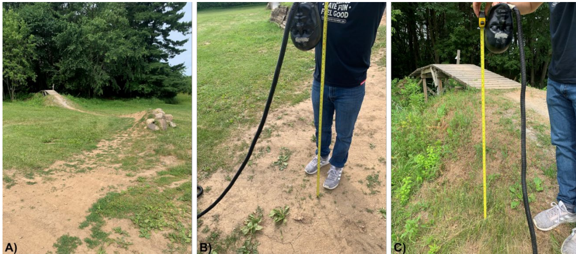
Fig. 1. A) Local MTB trails used for impact testing, B) Drop test setup for a normal impact onto a dirt surface, and C) Drop test setup for an oblique impact onto a 45-degree grass surface.
