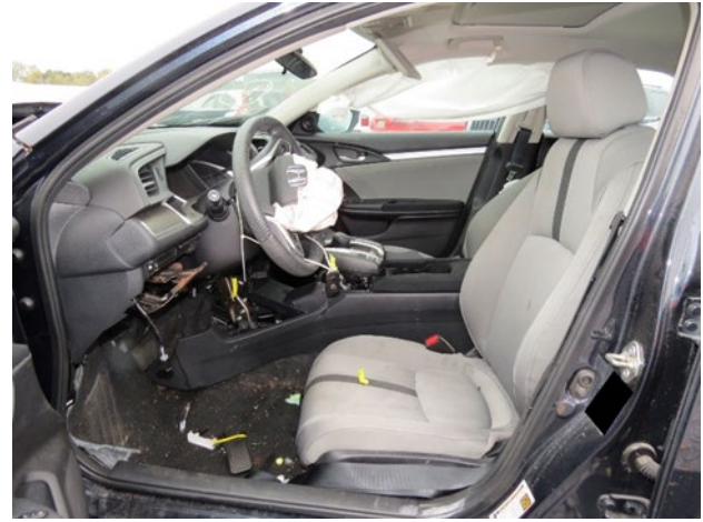
Fig. 13. Occupant's seating position in CIRENID 432, which was considered Exceedingly Severe based on the EDR-calculated speed change.
