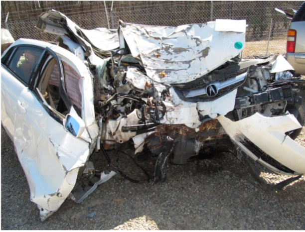
Fig. 12. Front crush for 2013-43-038-1-1 with high travel speed into a tree.
