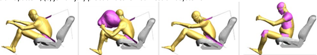
Fig. 3. In-crash motion postures of occupants with each restraint system.
