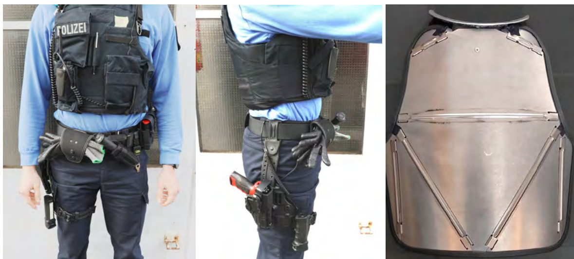
Fig. 1. Protective vest and police belt with accessories and thigh holster with pistol (left, centre). Sheet-metal inlay with "blade catcher" (right).
