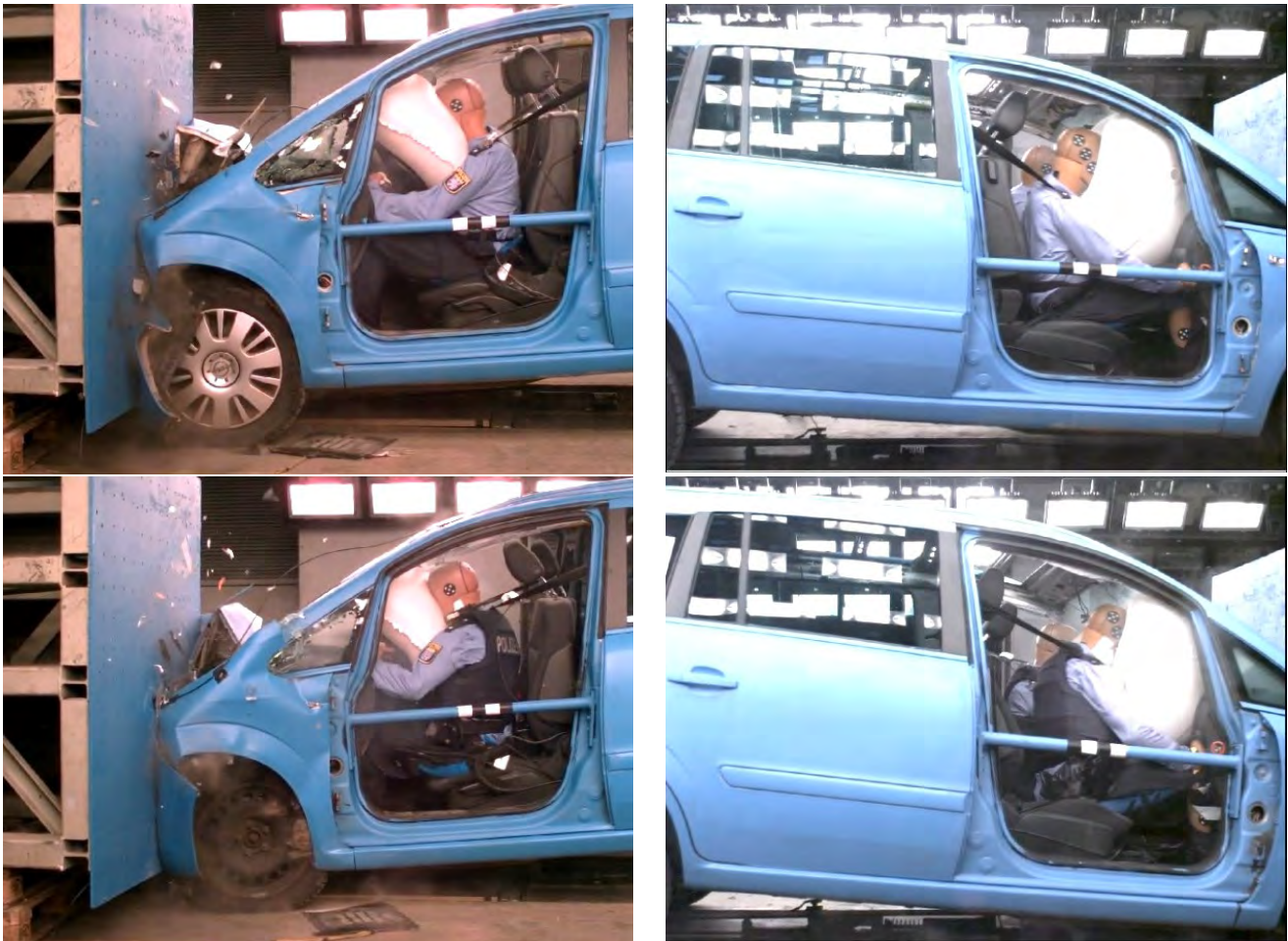
Fig. 4. Driver without PPE (upper left) and with PPE (lower left) and passenger without PPE (upper right) and with PPE (lower right), at time of respective maximum pelvis excursion.
