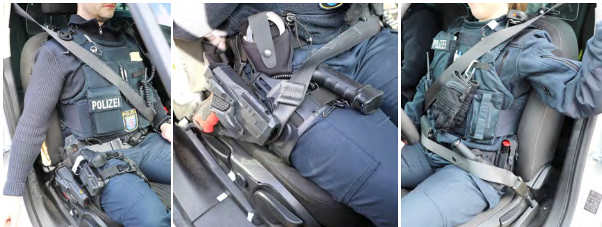
Fig. 8. Acceptable lap-belt path, outward shoulder-belt position (left), lap-belt under holster with extreme belt slack (centre), lap-belt over police belt and several accessories, acceptable shoulder-belt path (right).
