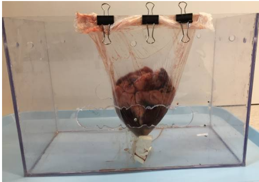
Fig. 1. Mounting apparatus of polycarbonate for the lamb heart.
