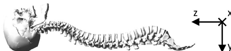
Fig. 1. The multibody model is composed of rigid bodies of the skull, vertebral bodies and sacrum. Adjacent vertebral bodies are connected by a 6 degree-of-freedom spring-damper element. Acceleration is input at the sacrum. The 3D representations of the skull and spine are for illustrative purposes and are not involved in the simulation. The coordinate system for the model is shown on the right.
