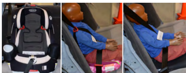
Fig. 5. Types of shoulder belt guide: fixed shoulder belt guide, flexible shoulder belt guide, free (left to right).
