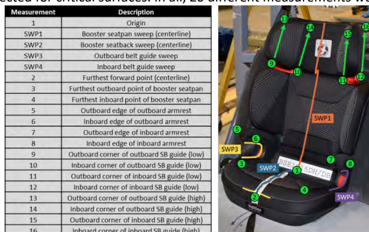
Fig. 3. Booster measurement points and sweeps.
