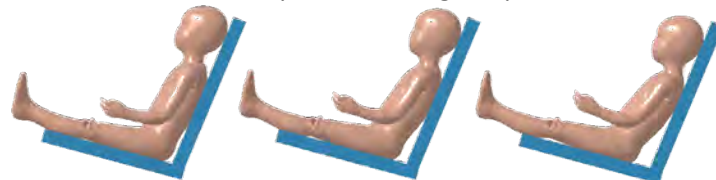
Fig. 8. HBM posture comparison. Upright posture, moderate slouch, and extreme slouch (left to right).
