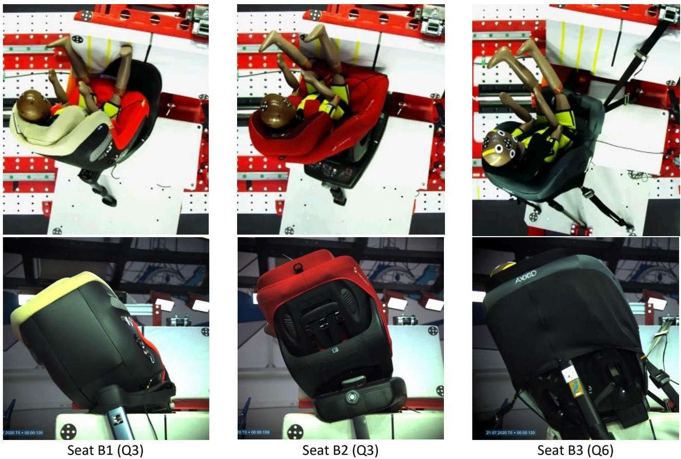
Fig. 2. Dummy and child restraint kinematics in rear-facing child seats.
