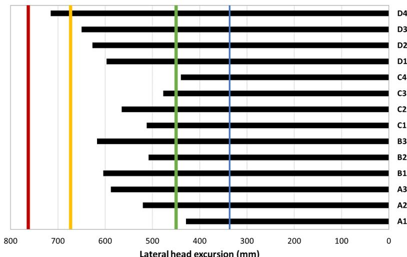
Fig. 5. Lateral head excursion from the centreline of the dummy’s seating position. Lines are marked to show the distances from the far-side seating position of a supermini car to the vehicle centreline (blue), child restraint interaction line (green), struck-side seat centreline (amber) and vehicle intrusion line (red).
