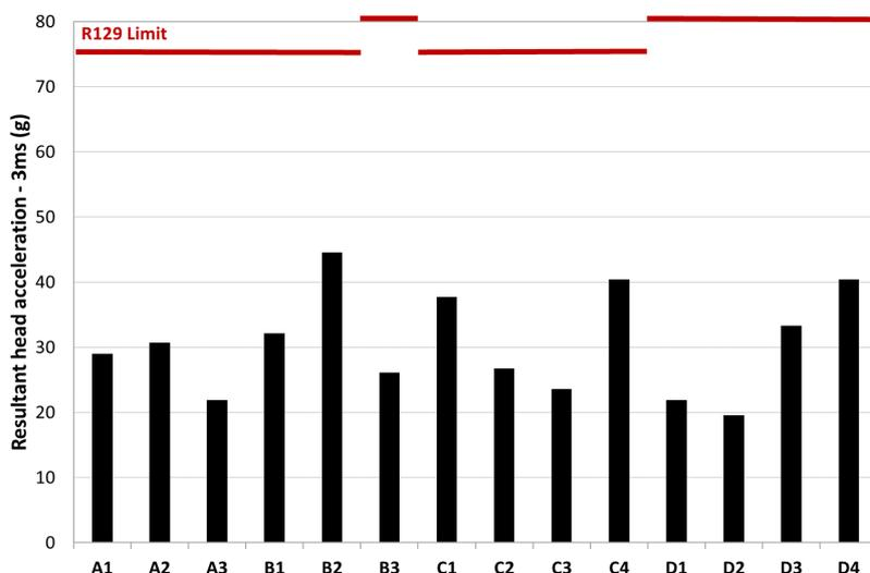
Fig. 6. Resultant head acceleration (3ms exceedance value) shown with the corresponding dummy limit in UN Regulation No. 129 struck-side impact test.
