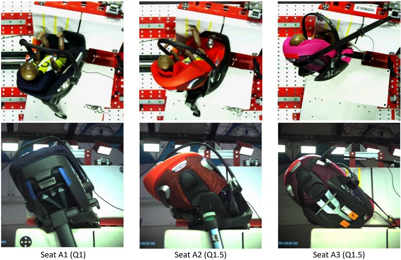
Fig. 1. Dummy and child restraint kinematics in infant carriers.
