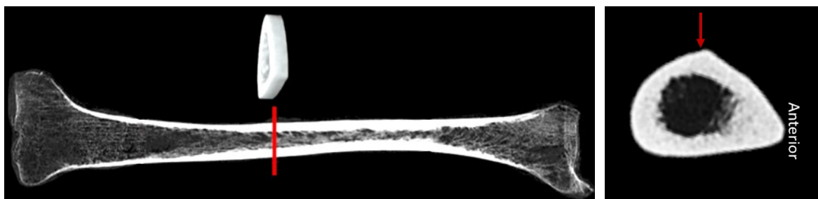
Fig. 1. Exemplar image of QCT scan with 50% volume of interest (VOI) designated with red line and inset image (left) and 50% cross-sectional image (right) with impact direction (red arrow).
