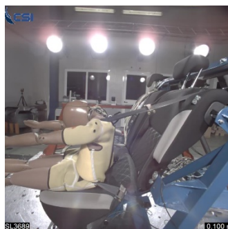
Fig. 2 Frame of the video at the time of maximum horizontal head excursion with seat belt alone (100 ms)
