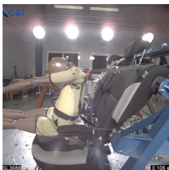
Fig. 1 Frame of the video at the time of the maximum horizontal head excursion with booster seat (106 ms)
