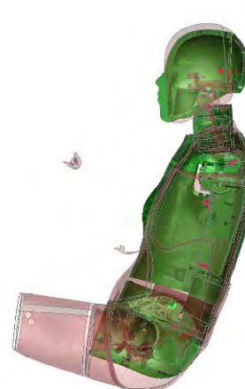
Fig. 2(b). Comparison of THOR-05F (maroon) and Hybrid III 5 th (green) positioning.
