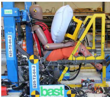
Fig. 1(a). The previous test setup with THOR-50M.
