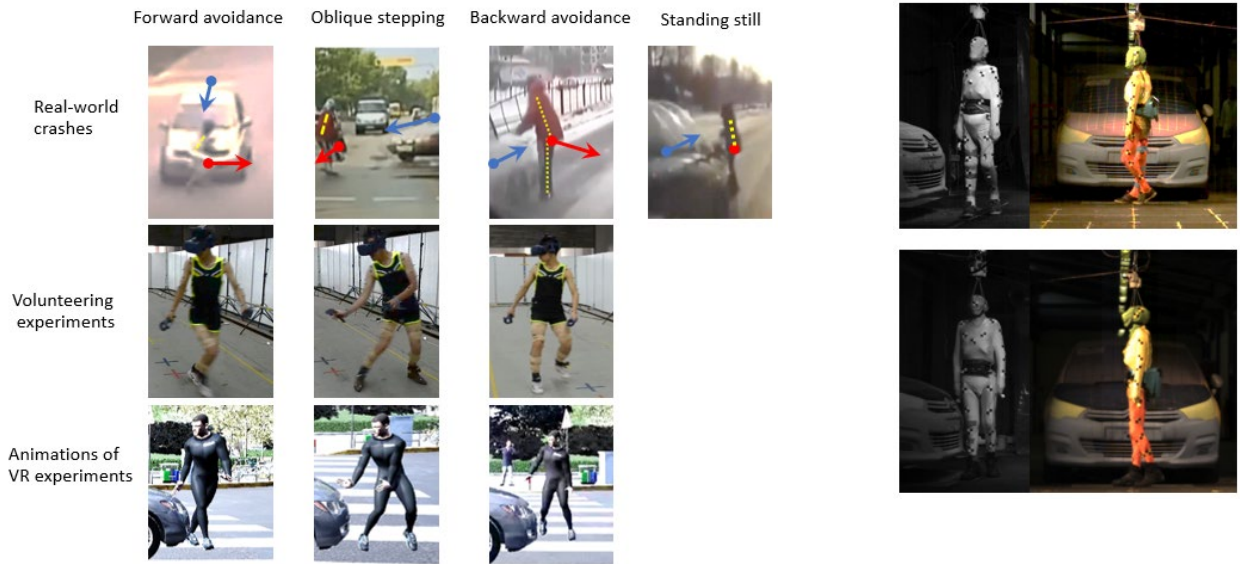
(a) Representative avoiding poses of pedestrians observed from real-world crashes and VR-based volunteering experiments
