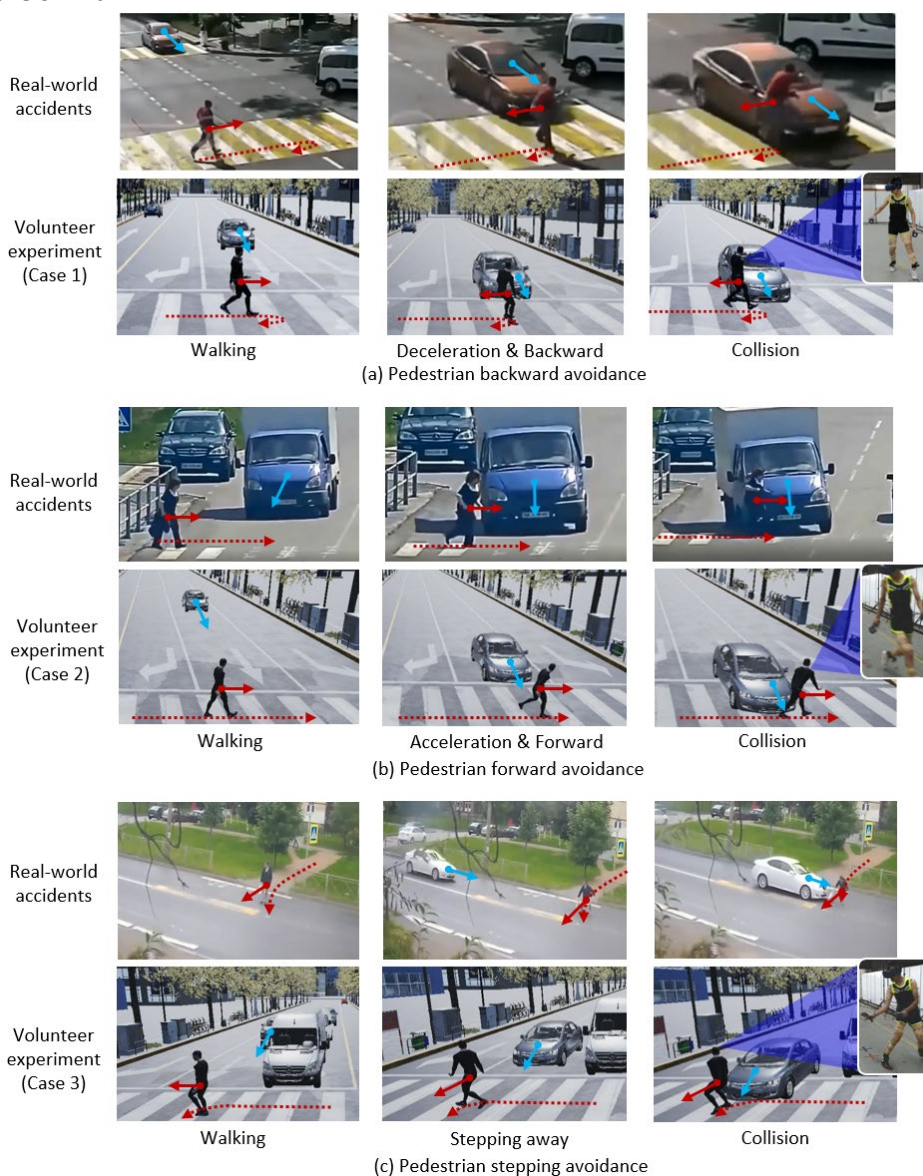
Fig. 2. Still shot of in vivo videos used to study pedestrian motion in car-pedestrian crashes. The red solid arrow and the dotted arrow represent the pedestrian’s moving direction and trajectory, respectively; the blue arrow represents the vehicle’s moving direction.
