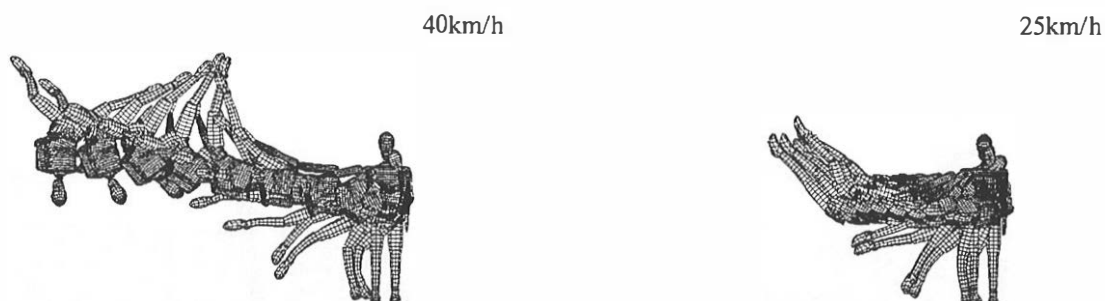
Figure 20 The influence of vehicle impact velocity at Y0 with deceleration and brake dive
