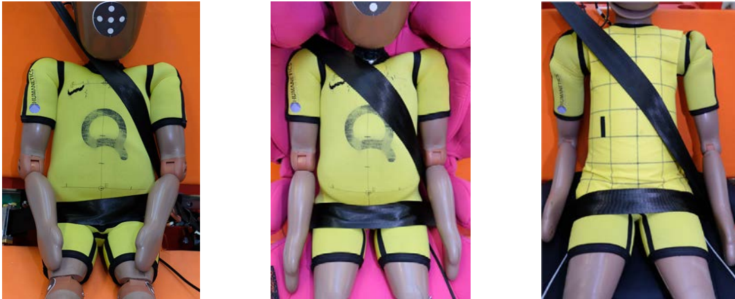
Fig. 12. Examples of initial static belt path, from left to right: Q3 with no CRS; Q3 in Seat 2; Q6 in Cushion 3.
