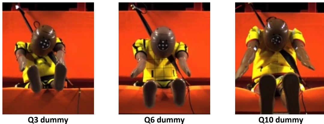
Fig.2. Dummy kinematics and belt interaction at peak head excursion with no booster.
