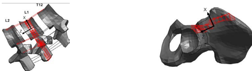
Fig. 7. Cross section definitions (in red) for lumbar spine vertebra L1 (left) and pelvis ASIS (right). Intervertebral discs not shown for the lumbar spine.
