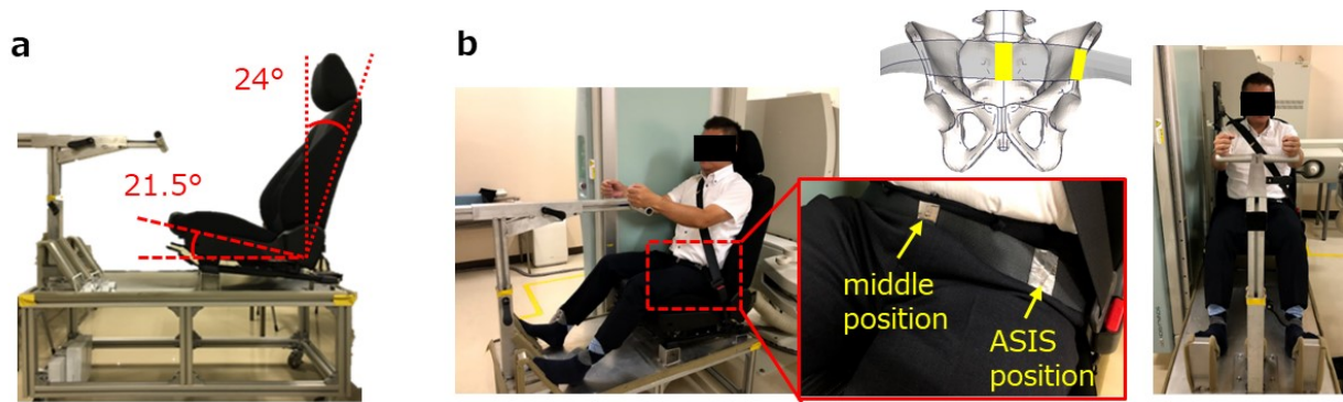
Fig. 2. The X-ray facility and situations of X-raying, a. the facility with an automotive driver seat, b. seated posture with the seatbelt.
