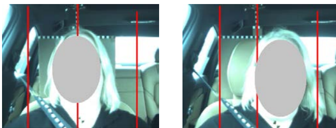
Fig. 4a. Example of sitting posture prior to turn (left) and at maximum lateral position (right); shorter participant in TurnC, inboard.
