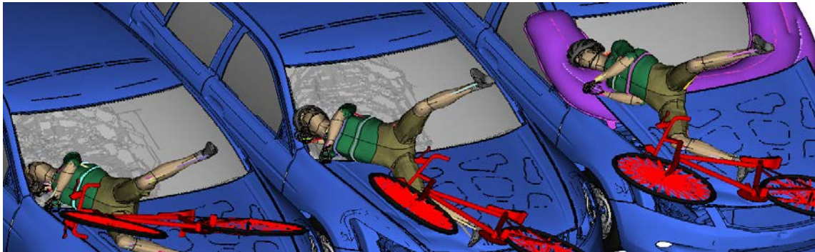
Fig. C2. Snapshots from impact between vehicle velocity 40km/h and bicyclist moving in 15km/h, at time of head impact.
