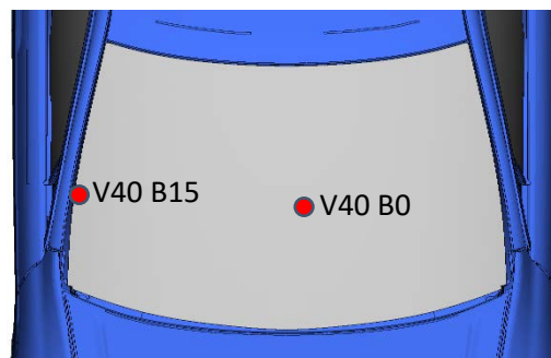
Fig. 4. Approximate head impact points on windscreen for all impact configurations. “V” indicates vehicle velocity and “B” bicycle velocity (km/h)
