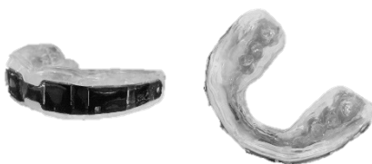
Fig. 1. The Prevent Biometrics IMM mouthguard with instrumentation along the teeth.
