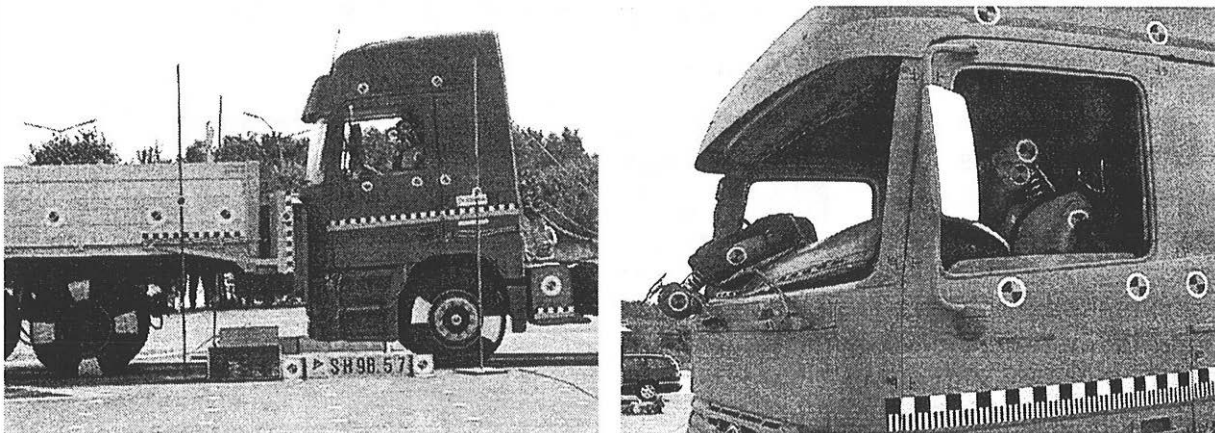
Fig. 3: Impact constellation and final position of the driver and co-driver dummy
