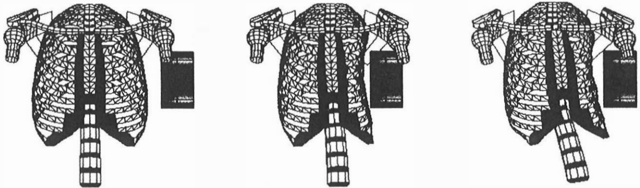
Figure 6: Lateral Impact simulation on the thorax, configuration 9, time 0, 20 and 40ms
