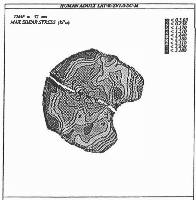
Fig. 14 Shear stress contours at 32 ms: lateral rotation, coronal section in the forebrain.
