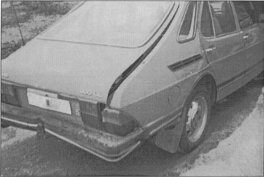
A common deformation of a rear-end impact where the occupant/ occupants sustain an impairment to the neck AIS 1.
