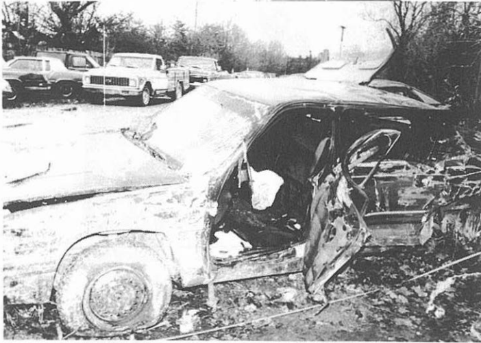
Fig. 7 Side swipe type of crash. Wrist and hand fractures from instrument panel impact due to deploying air bag.
