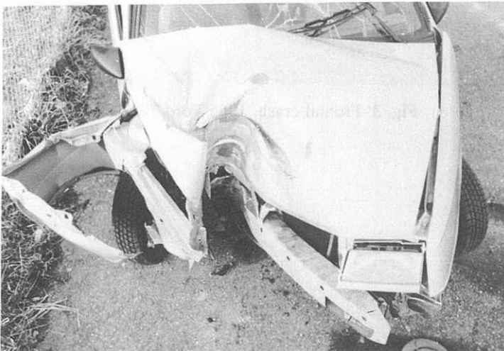
Fig. 5 Frontal crash into a tree, 1991 Dodge Shadow
