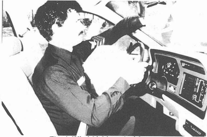
Fig. 4 Windshield cracked from hand impact due to air bag deployment.
