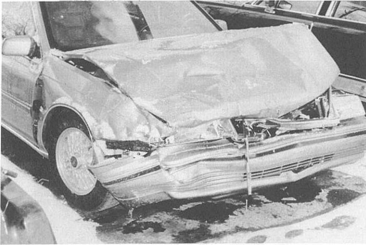
Fig. 10 1990 Lincoln Continental with frontal damage. Airbag deployment flung the driver's right hand to the instrument panel producing a wrist fracture.
