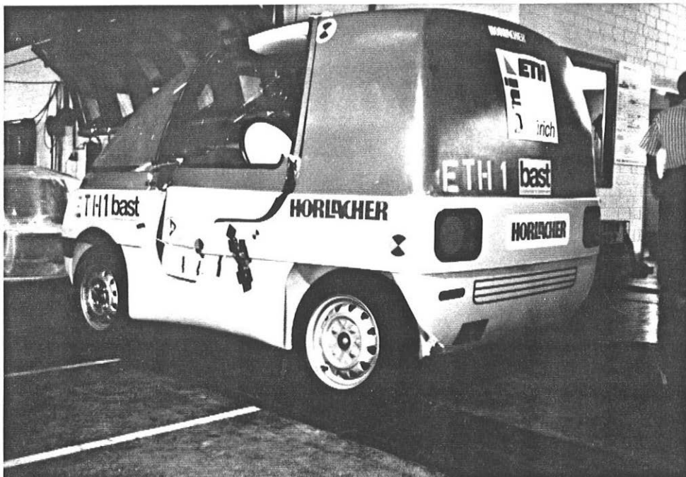
fig 5 Damage of the "impact belt" vehicle after side impact with the European barrier at 50 km/h
