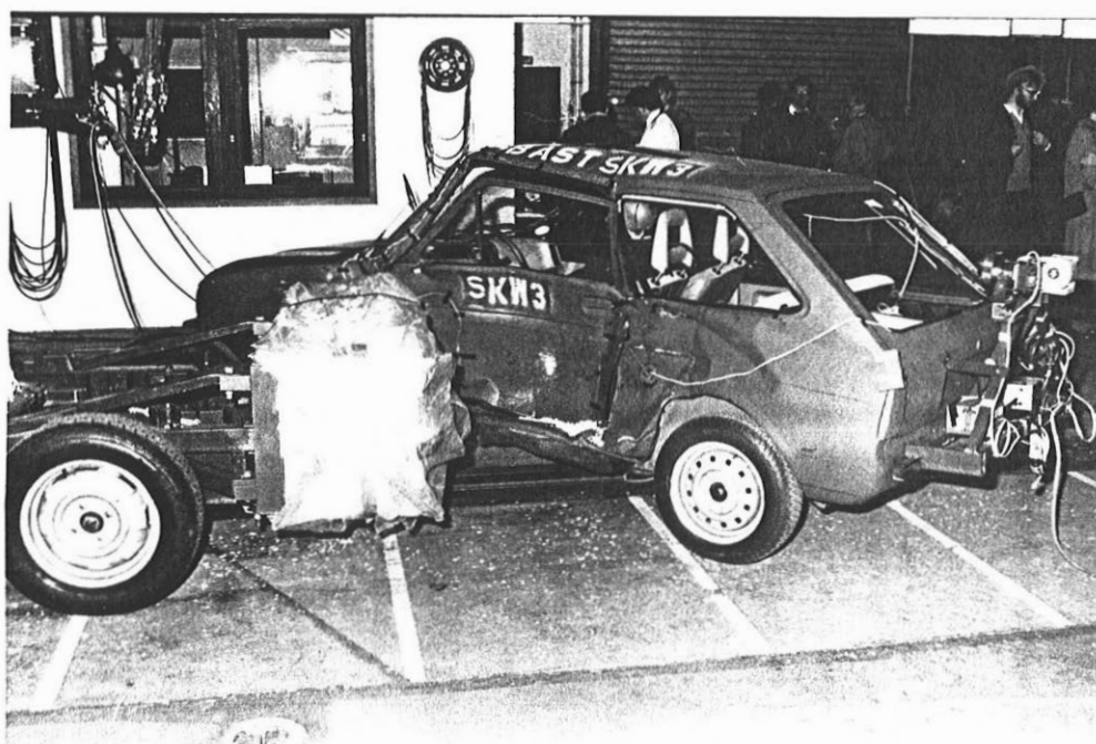
Fig A.1 : Final Position and Deformation Picture in the Tests with a Ford Fiesta
