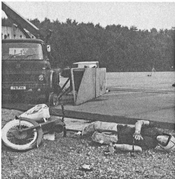
FIG.3 MOTORCYCLE AND DUMMY ARRESTED IN GRAVEL
