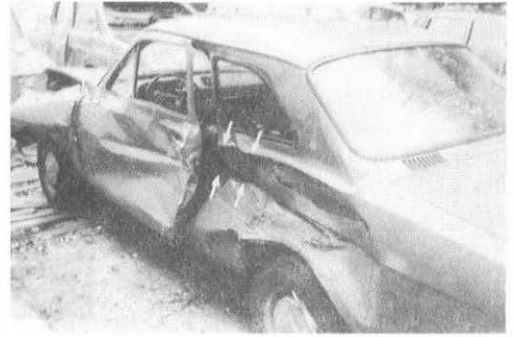
Figure 14: Deformation Characteristic Dependent on Truck Size
