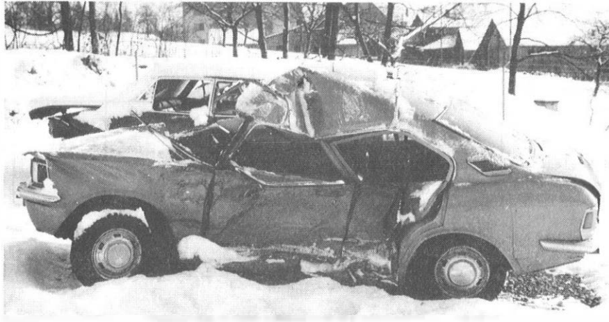
Photo No. 3 : Usually the B-pillar is also displaced towards the middle of the car. No "compression" between belt and intruding structure occurs.
