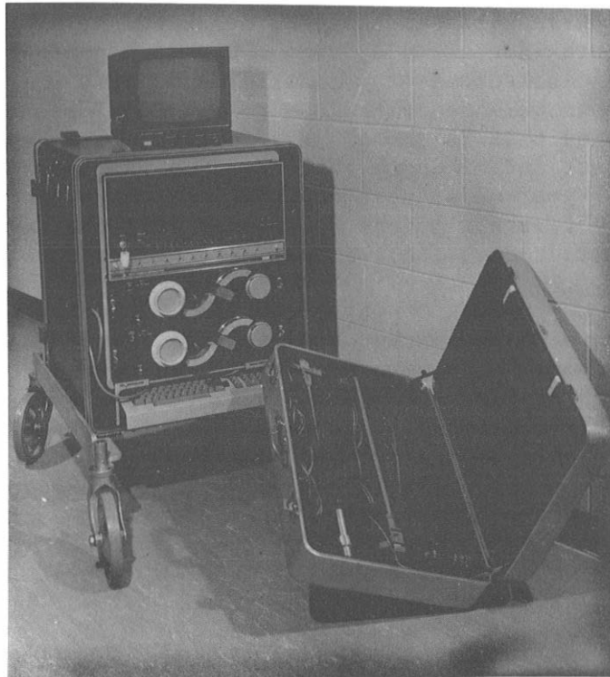
Fig. 1. The complete mini-computer (NOVA 1220) anthropometric system is designed for portability. The case on the right carries all measuring instruments, and the keyboard, terminal, and complete data acquisition system is contained on the left.
