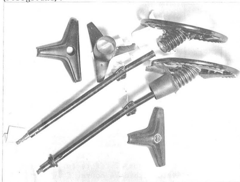
FIGURE 2. A damaged "deformable can" system, removed from a Ford Capri, showing bending of can and column with little damage to the wheel rim and spokes. (Background). Similar damage produced under modified test conditions. Column angle used was 10^{\circ} more than normal installation angle (Foreground).
