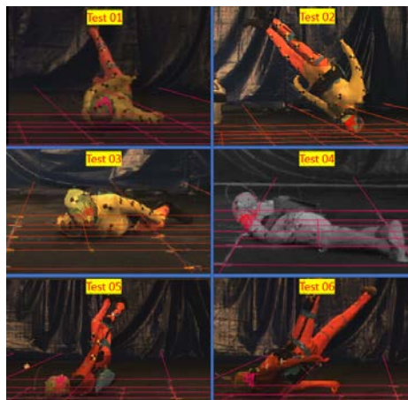
Fig. 2. Still shots of head ground contact with MBIM fit at instant of ground contact.
