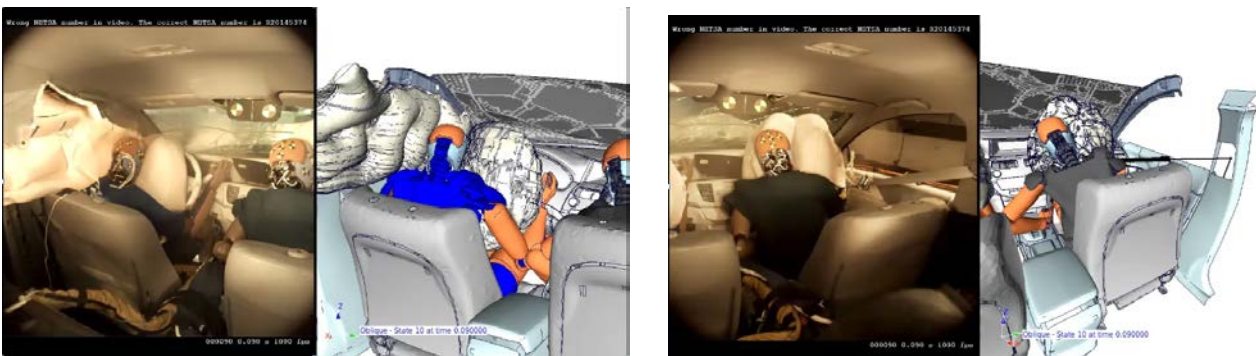
Fig. 3. THOR Kinematics in Test and Simulation (a) Near-Side, (b) Far-Side.
