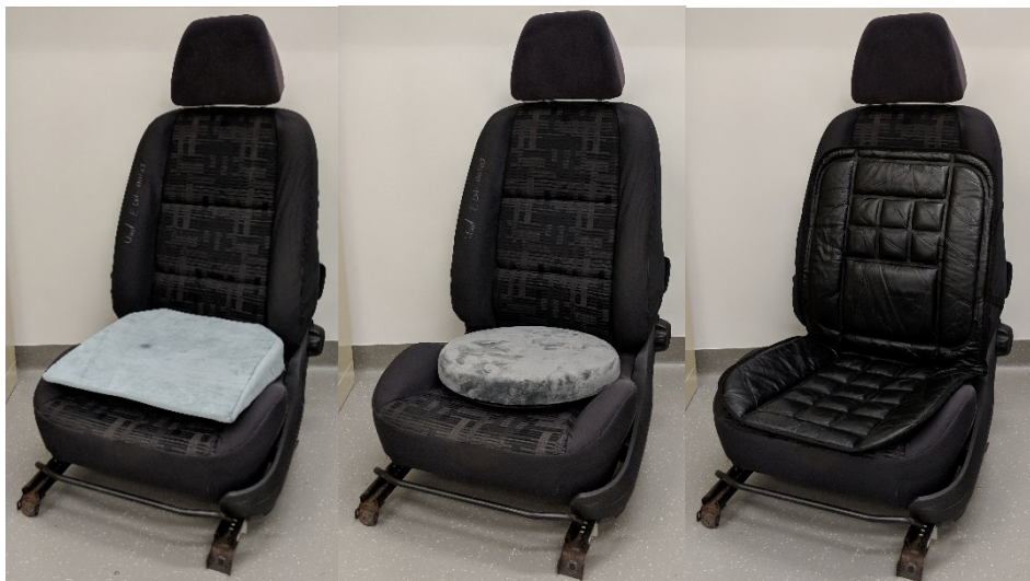
Fig. 1. Tested comfort accessories: Seat wedge cushion (left), swivel seat cushion (centre), padded seat cover (right).
