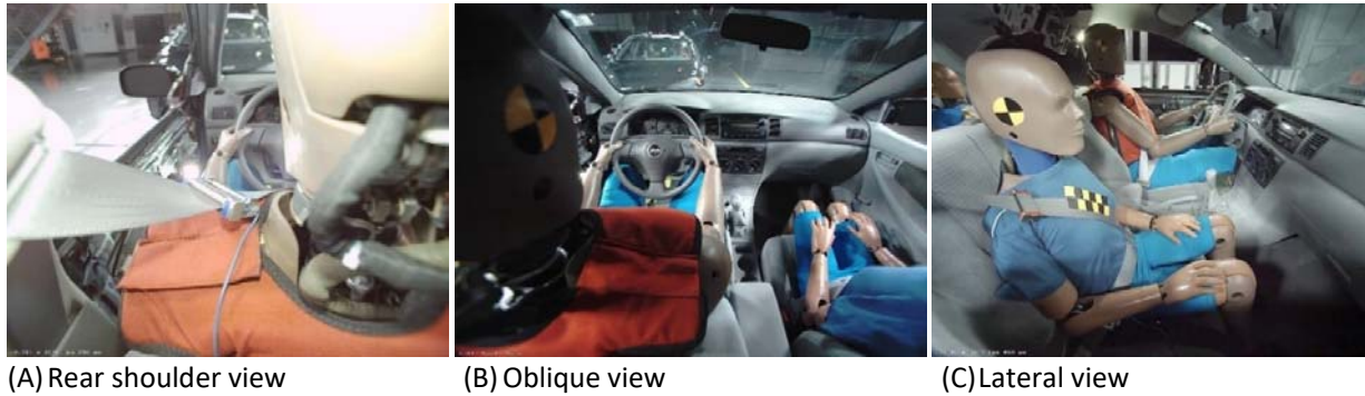
Fig. 9. Camera views of THOR ATD in driver position.
