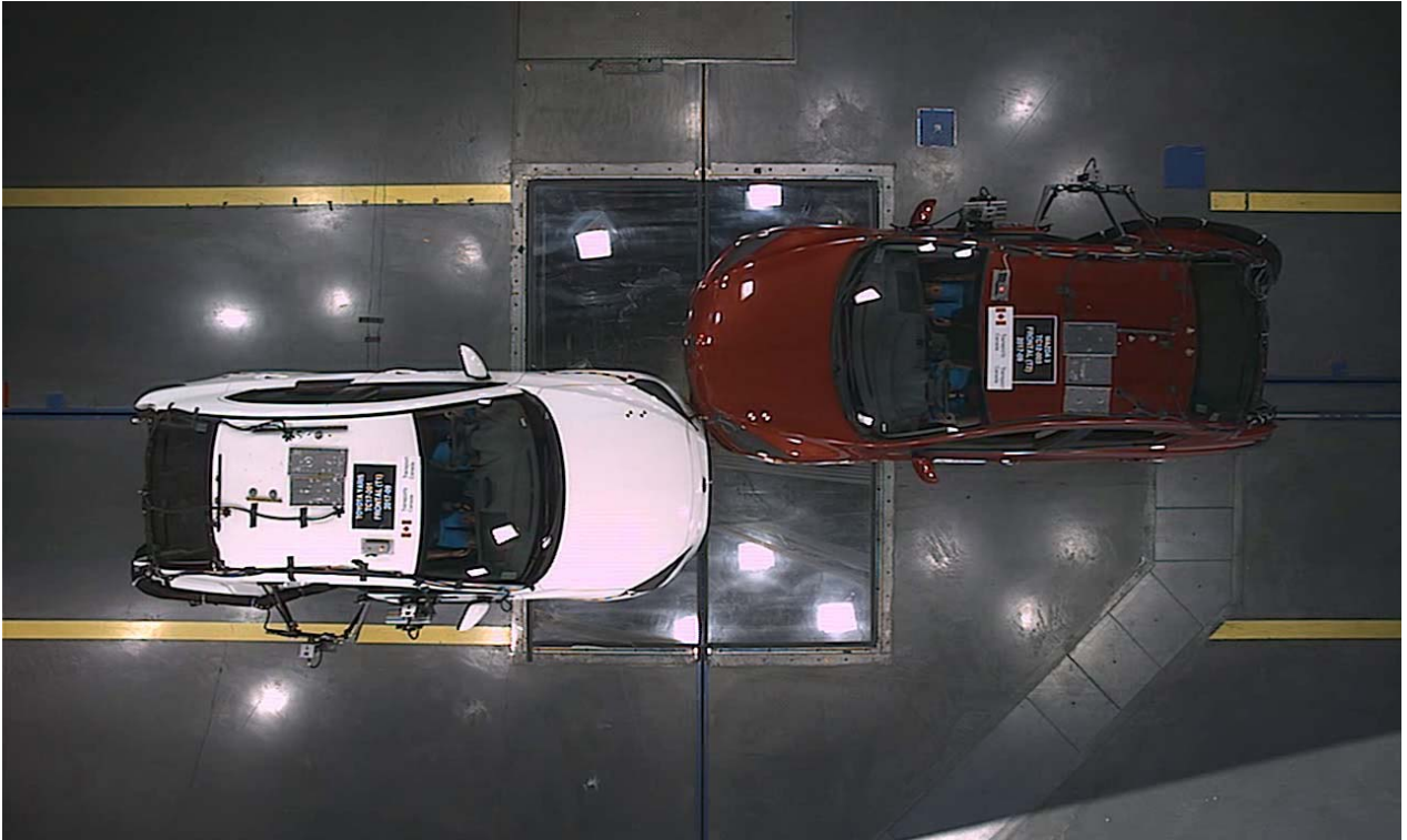
Fig. A1. Top view of a 40% offset configuration
