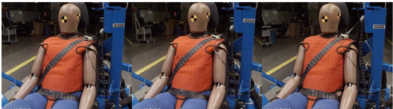
(A) Position 1 distal from the neck (B) Position mid-way (C) Position 5 proximal to the neck Fig. 5. Photos of seatbelt placement and D-ring positions for the sled tests.
