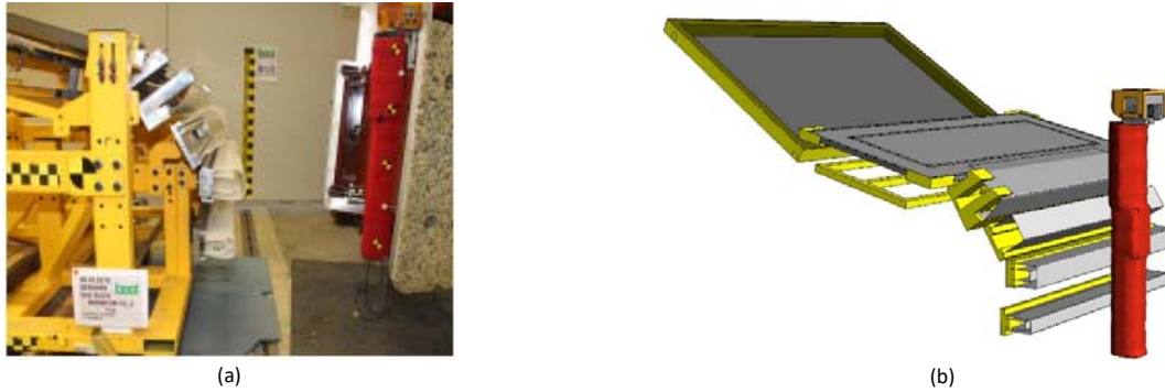
Fig. 2. SAE buck test condition for the FlexPLI-UBM hardware (a), and FE model set up (b).
