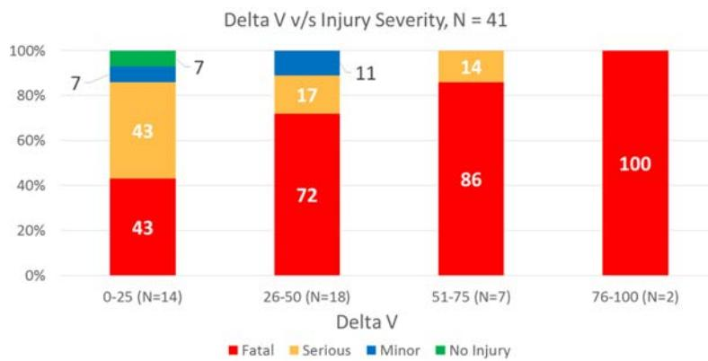
**Fig. 9. Delta V vs Injury Severity of passenger car distribution.**
