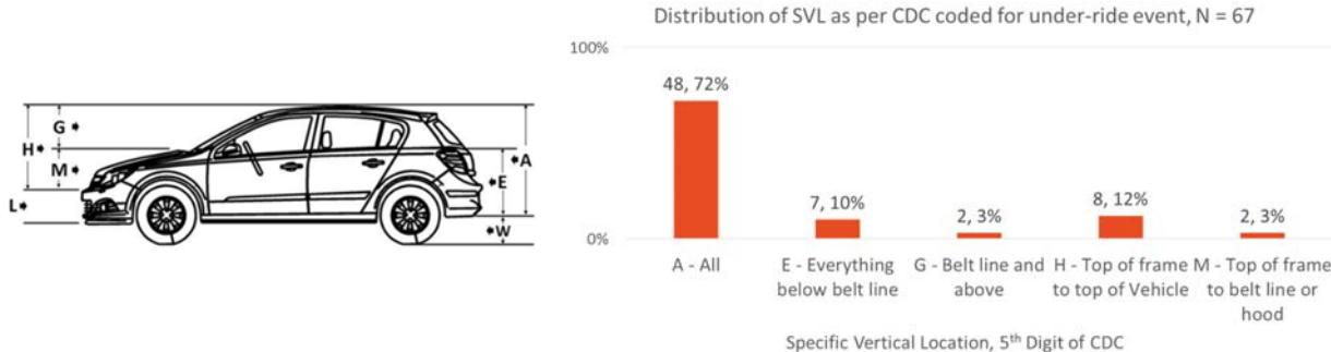
**Fig. 2. Distribution of Specific Vertical Location of the CDC for the under-ride event of the passenger cars.**
