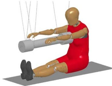
Fig. 2. THOR-5F Thorax Probe Impact Model Set-up.
