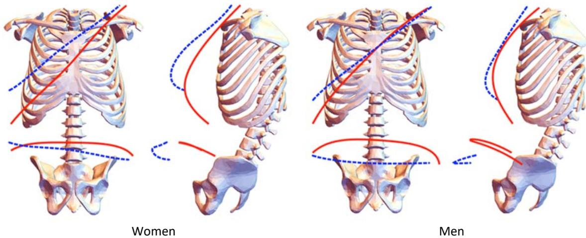
Figure 5. Mean belt paths for low (—, 30 kg/m<sup>2</sup>) and high (---, 55 kg/m<sup>2</sup>) BMI for men and women with mean stature (M=1630 mm, F=1750 mm) relative to scaled midsize-male skeleton.
