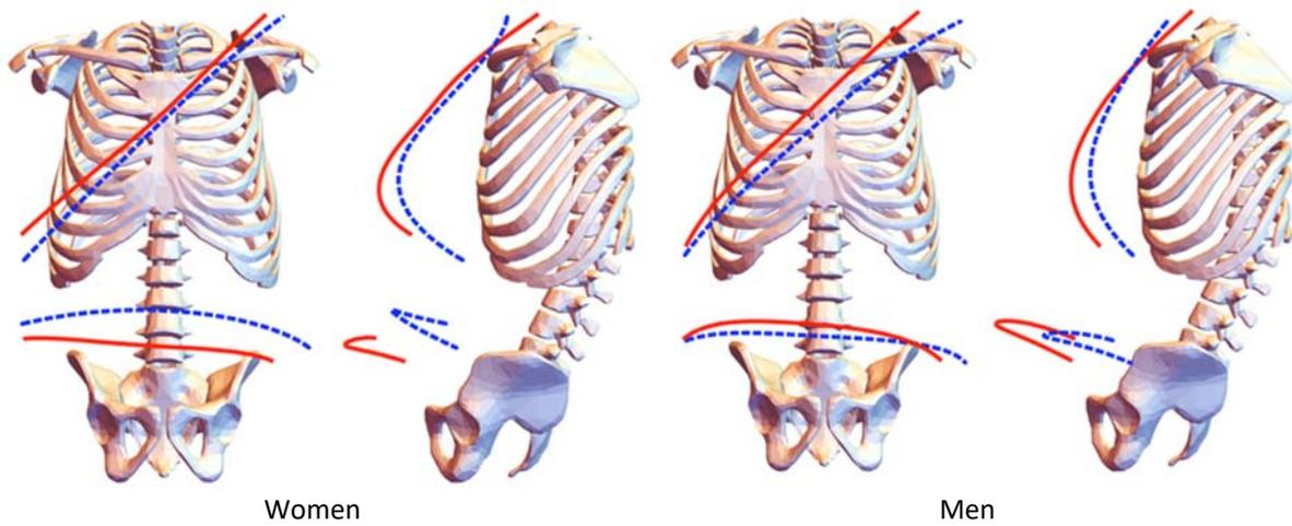
Figure 4. Mean belt paths for short (—, M=1600 mm, F=1500 mm) and tall (---, M=1870 mm, F=1750 mm) stature for men and women with BMI=40.5 kg/m<sup>2</sup> relative to scaled midsize-male skeleton.
