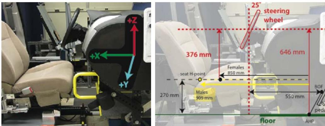
Figure 1. Vehicle mockup and package dimensions for mid-sized sedan condition.
