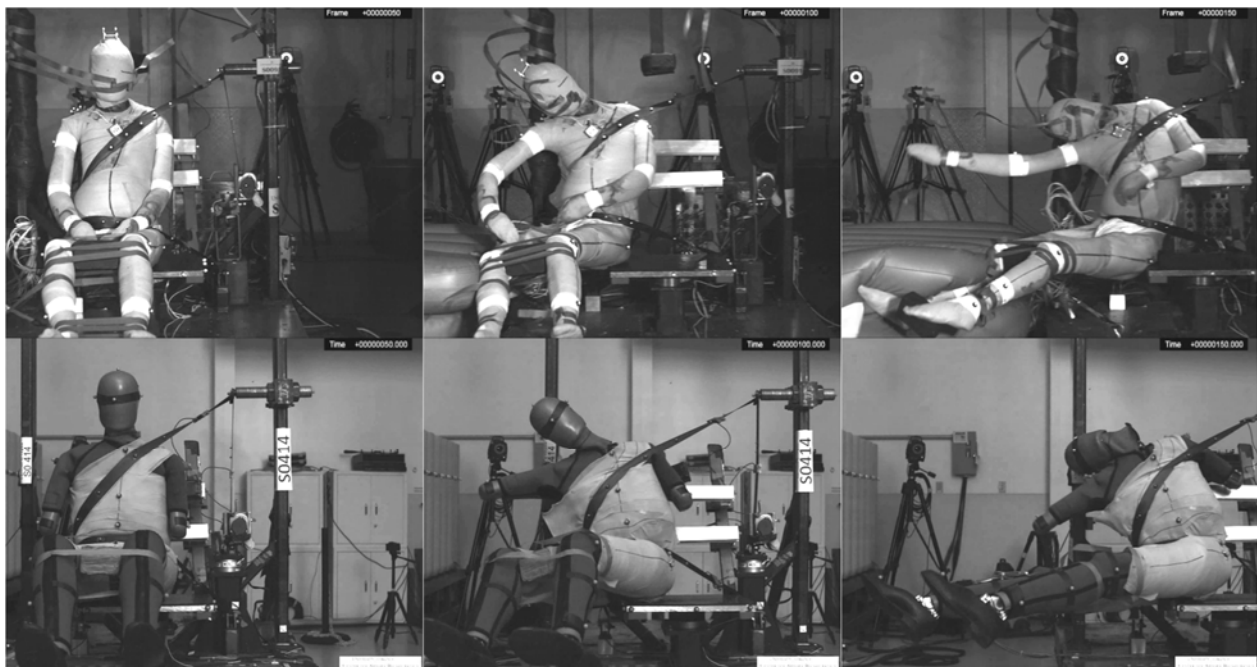
Fig. 2. WorldSID vs PMHS comparison in lateral impact configuration at 50 ms (left), 100 ms (center) and 150 ms (right).
