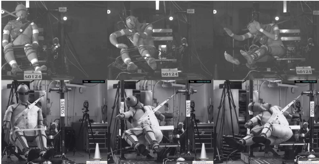
Fig. 1. WorldSID vs PMHS comparison in oblique impact configuration at 50 ms (left), 100 ms (centre) and 150 ms (right).
