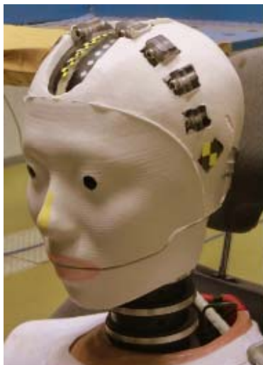
Fig.4. Assembled Dummy Head mounted on Hybrid III neck
