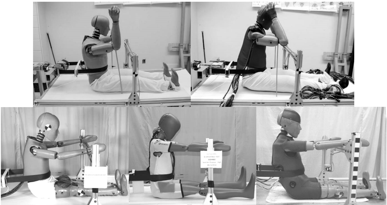
Fig. 2. Pre-test positions of HIII-50M (top left), THOR-K (top right), HIII 10yo (bottom left), Q10 (bottom center), and LODC (bottom right).
