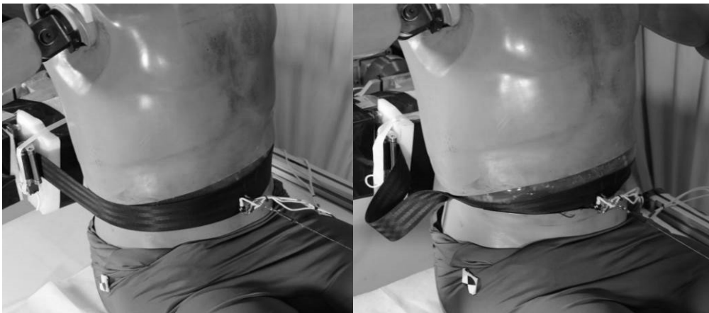
Fig. 7. Initial placement of seatbelt on the Hybrid III with RRSA (left); final position of seatbelt trapped between the chest jacket and pelvis (right)
