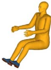
Fig. 3. Whole human body finite element model.
