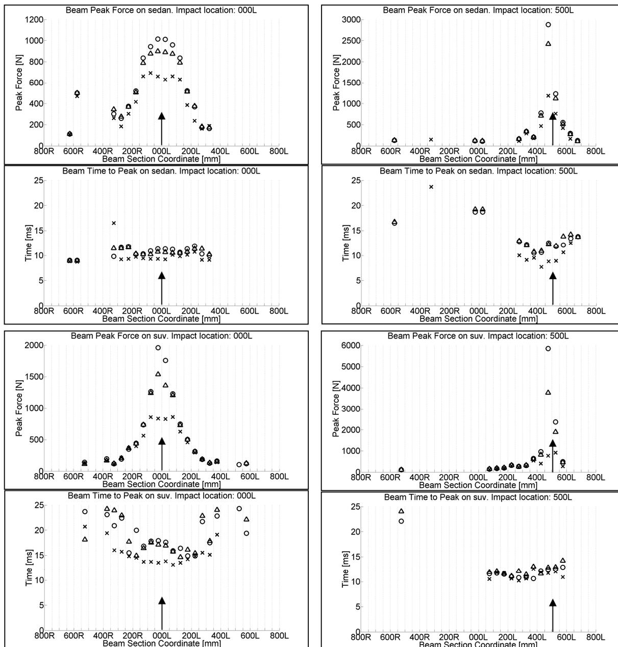
Fig. 1: Force information for THUMS (x), Flex-PLI (o) and Flex-PLI at Euro NCAP position (Δ) with an arrow representing the impact location
