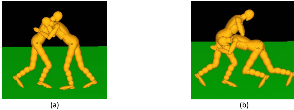
Fig. 2. The multibody player-to-player configuration for an (a) Upper Body Tackle and (b) Lower Body Tackle.
