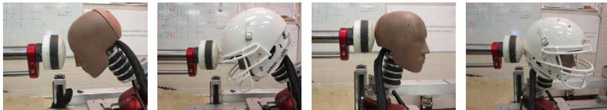
Fig.1a) Bare Front PE Fig.1b) Helmeted Front PE Fig.1c) Bare Rear Boss CG Fig.1d) Helmeted Rear Boss CG Fig.1: Bare and Helmeted Impact Set ups – Example for Front Positive Elevation (PE) and Rear Boss Center of Gravity (CG)
