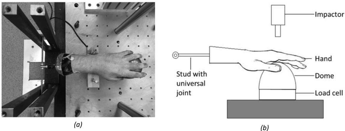
Fig. 1. Experimental set-up at the drop tower. (a) Photograph from the top. (b) Schematic of the set up from the side.
