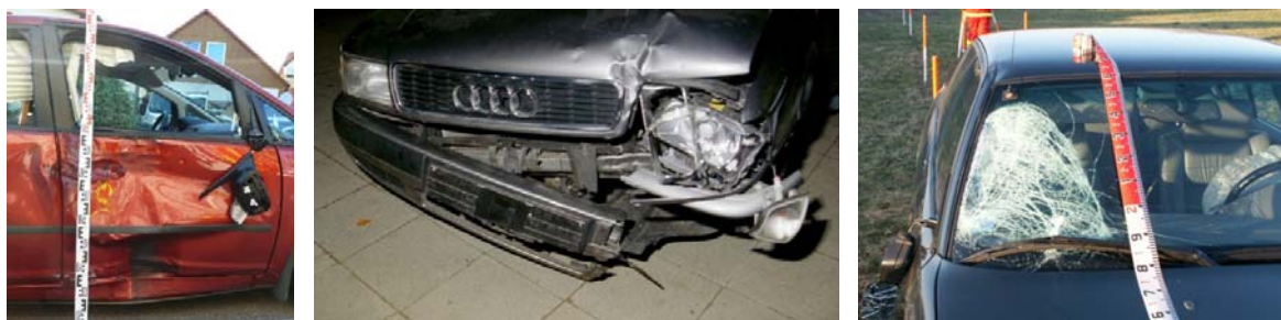
Fig 9. Case examples of car injury sources: Car side low, Car front low, Car windshield (from left to right)
