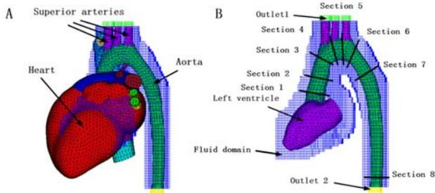
Fig. 1. FE model depicting different components and the location of each aortic section
