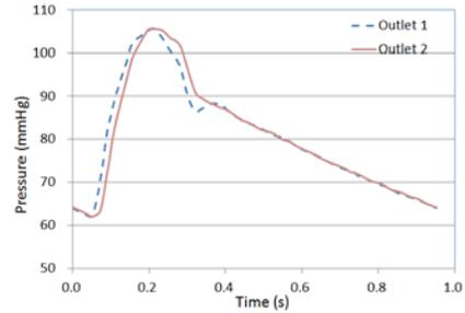
Fig. 2. Boundary conditions of time-dependent pressure for outlet 1 and 2
